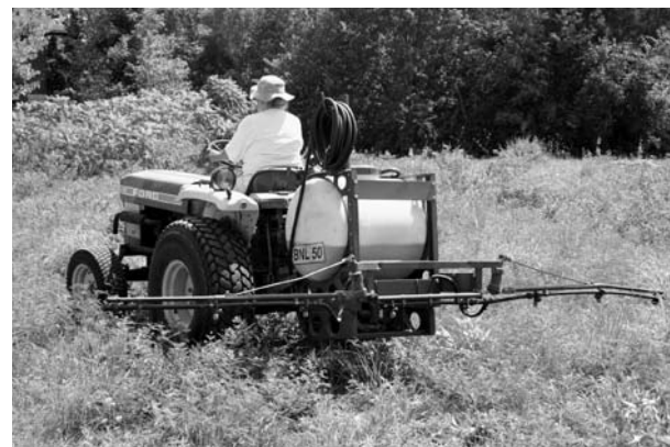
Top: Various size herbicide sprayers. Bottom: Fifty-gallon spray rig with a 15-foot boom is practical for sites larger than a half acre.
